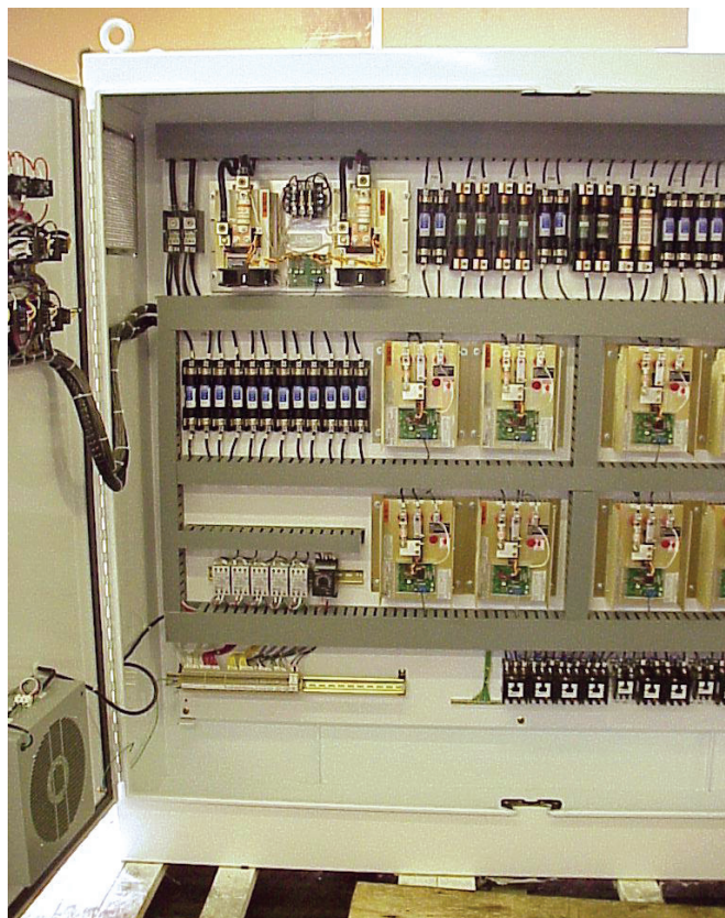
SCR power control safety design features. The SCRs have I 2 T fusing and MOV voltage protection, and heat sinks are spaced at a safe distance from each other for efficient cooling. Door mounted fan and vents in top of enclosure provide sufficient cooling for all components. Courtesy of Radiant Energy Systems.
